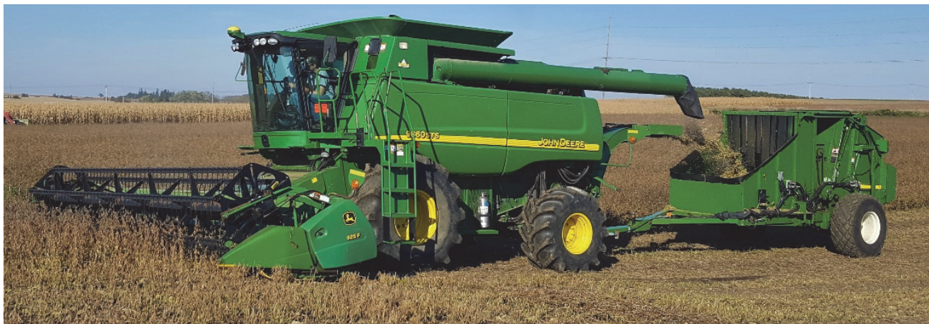
Figure 1. Single-pass round baler (SPRB) collecting material exiting the combine harvester residue chopper during soybean harvest.
