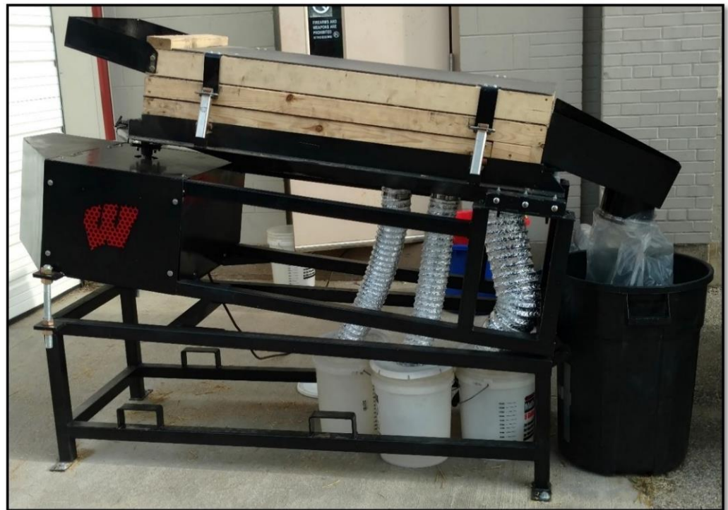
Figure 3. The gyratory screener with the fraction collection containers.
