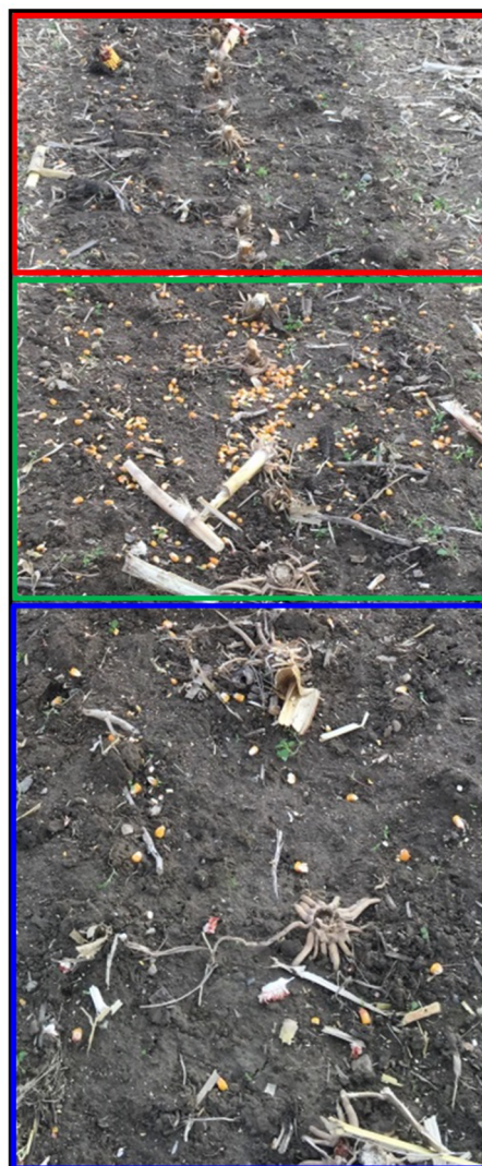
Fig. 7. Spatial variability in kernel loss after harvest with corn header using 44 mm deck plate spacing after one residue clearing operation (Experiment No. 4). Note that kernel loss is moderate (blue outline); then heavy (green outline); then light (red outline).
