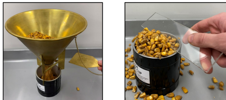
Figure 1. Grain emptying into container from discharge funnel (left). Leveling the contents with straight edge per USDA standard instructions [17] (right).
