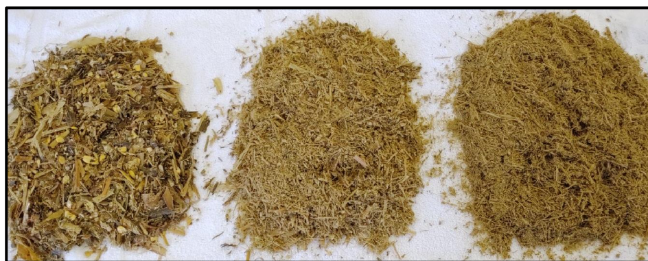
Figure 2. Whole-plant corn (after ensiling) processed with an on-board kernel processor (left—KP treatment) or with the experimental processor either once (middle—1X treatment) or twice (right—2X treatment). Processing took place prior to ensiling.
