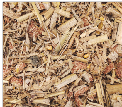
Figure 1. Typical example of MOG and grain mix that was delivered to cleaning system.
