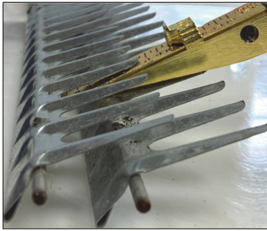
Figure 5. Measuring sieve clearance between adjacent rows of sieve louvers using a tapered wedge scale.
