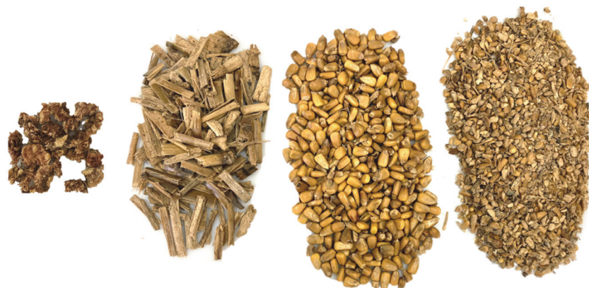
Figure 6. Typical material located in the Separated Grain. From left to right, cob pieces, stalk rind and pith, whole grain, and broken grain. All material to the same scale. The two left hand materials were typical examples of Foreign Matter (FM) found in the Separated Grain.
