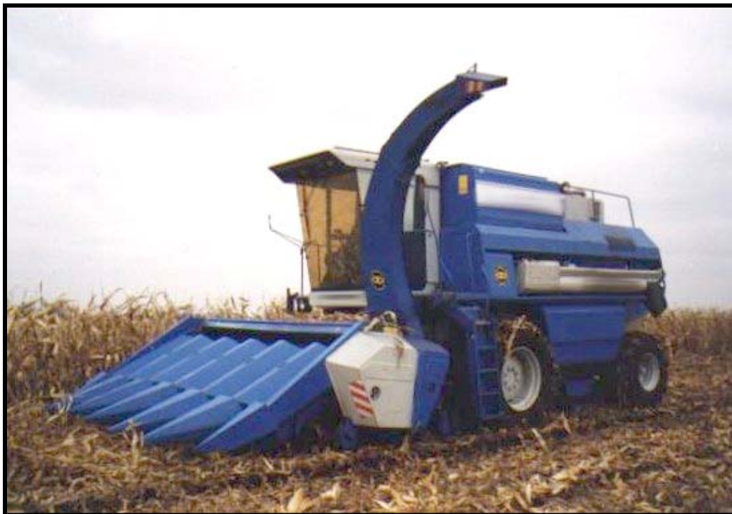
Figure 3. Modified combine crop unit used to chop and blow leaf and stalk fraction from harvester during grain harvest.
