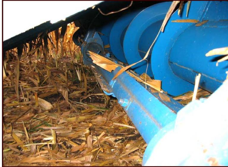
**Figure 3.** Knife rotor used to gather and size-reduce the stover ejected from the snapping rolls of the stalk-gathering head.
