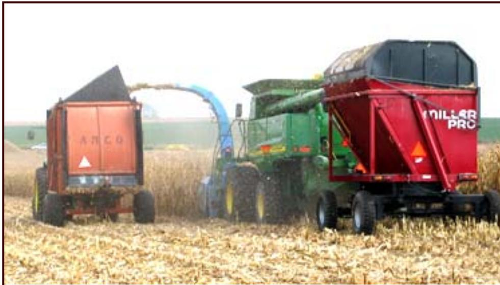
**Figure 4.** Modified grain combine harvester with stalk-gathering head, collecting stalk and leaf in front wagon and cob and husk in rear wagon.
