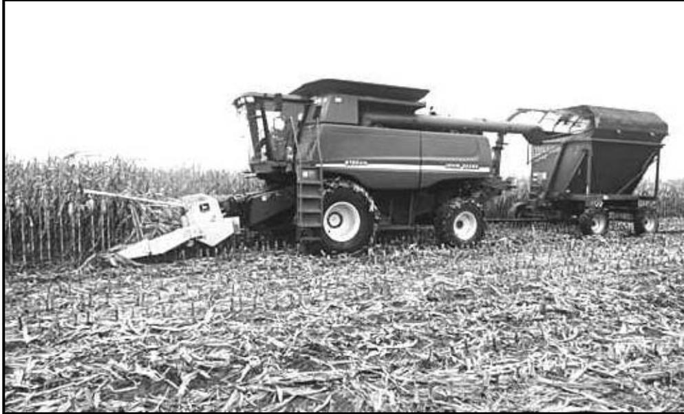
***Figure 1.*** Modified grain combine with whole-plant forage harvester corn head. *Photo courtesy of Wolfgang Hoffman.*
