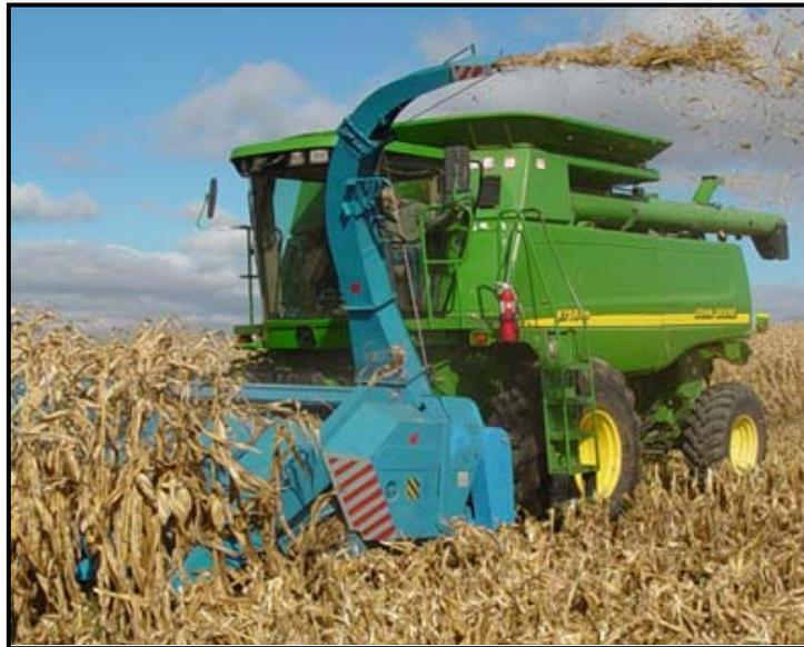
***Figure 2.*** Modified grain combine harvester with stalk-gathering head to gather, size-reduce and transport the stalk and leaf fractions at the head
