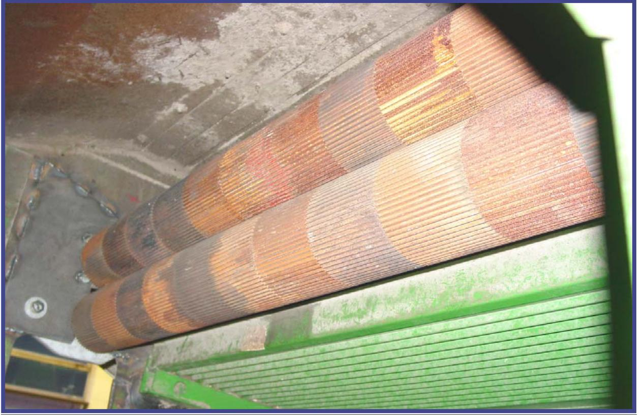
***Figure 5.*** Crop processing rolls at exit of cylinder discharge beater.
