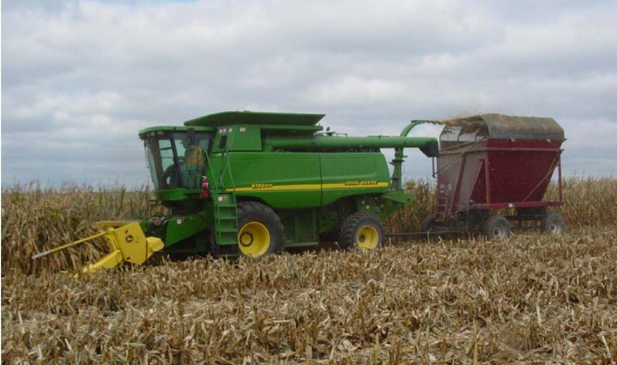
Figure 2. Single-pass stover and grain harvester used for October 20, November 3, 4 trials.
