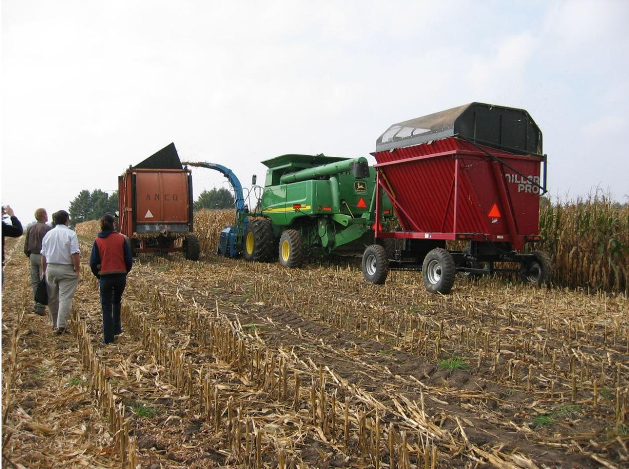
Figure 1. Single-pass stover and grain harvester used for the October 11 trial.
