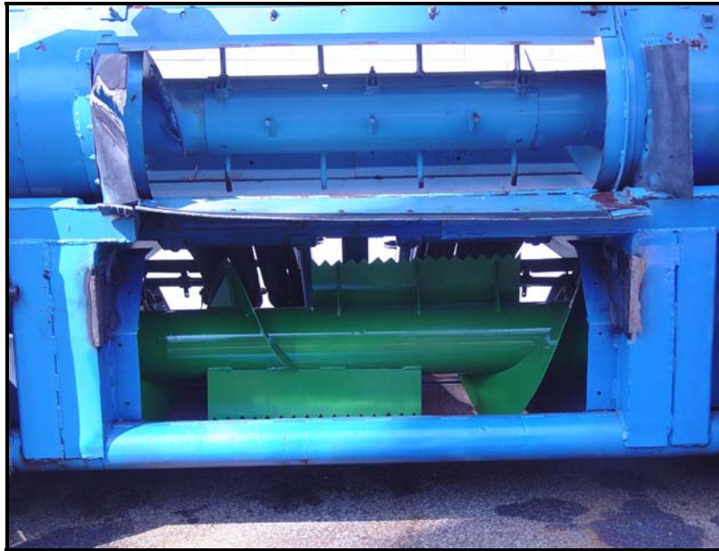
Figure 3. View from rear of stalk-gathering head showing discharge for the ear gathering auger (top) and discharge of stalk gathering auger (bottom). Ears were fed into the combine feederhouse and stalks were formed into a windrow on the ground underneath the feederhouse.
