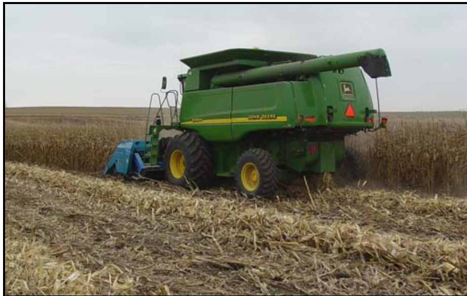
Figure 2. Combine harvester configured to harvest stover in single-pass using precision-cut stover processor (top) or to harvest stover in two-passes by forming stover windrows during grain harvest (bottom). Note that MOG exiting the rear of the combine was placed on top of the windrow formed by the stalk-gathering head.
