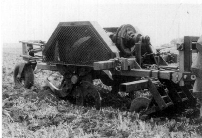
Fig. 2. Active-passive tillage machine
