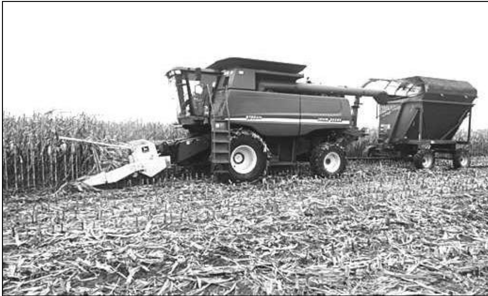
Figure 1. Modified grain combine producing single-pass, split-stream harvest of corn grain and stover. Photo courtesy of Wolfgang Hoffman.
